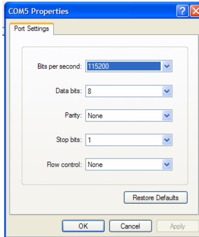
Figure 1. KlasRouter HyperTerminal COM Port Settings Window
